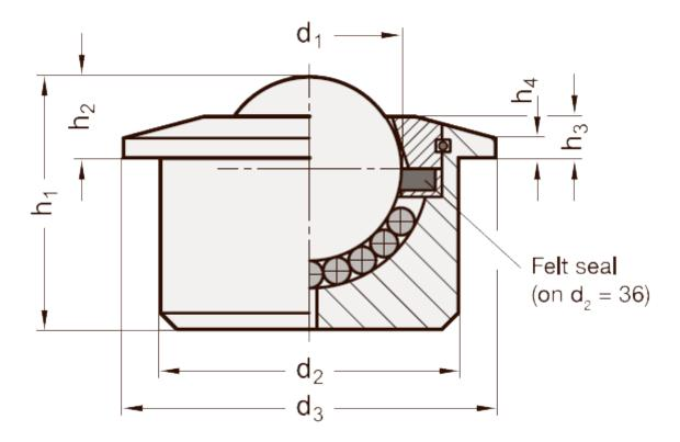
$$\begin{array}{lll} d1 & = 30.1 \\ d2 + / -0.08 & = 45 \\ d3 & = 55 \\ h1 + / -0.3 & = 36.8 \\ h2 + / -0.3 & = 13.8 \\ h3 + / -0.3 & = 7 \\ h4 & = 4.5 \\ Max load (N) = 2000 \end{array}$$
